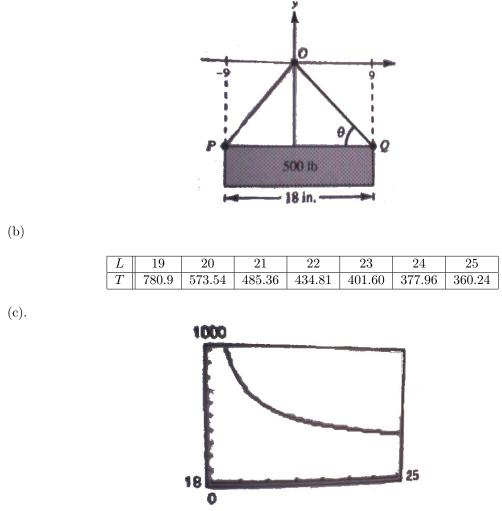
(d). The line T = 400 intersects the curve at L = 23.06 inches. (e).  $\lim_{L \to \infty} T = 250$ . The maximum tension is 250 pounds in each side of the cable since the total weight is 500 pounds.
